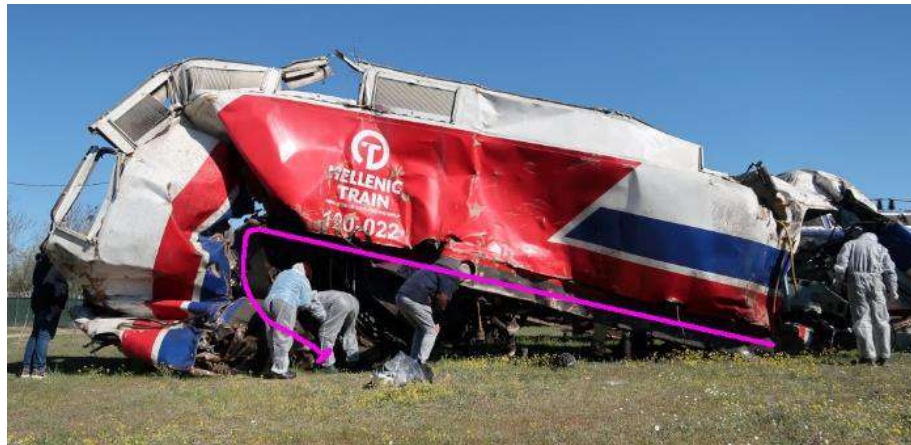
Figure 14. The first locomotive of the freight train (120-022) showing extreme damage from the very heavy head-on collision with the locomotive (120-023) of the passenger train.
