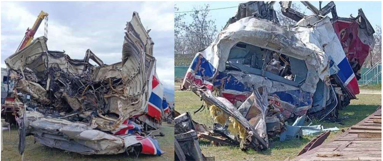
Figure 77. Position 1) Siemens Hellas Sprinter 120-022- NVR Engine: 91 73 212 0 022-7 Extreme damage on the front, roof missing, and rear heavily damaged from the rear collision with the attached locomotive 120-012. Rear view in Figure 14.
