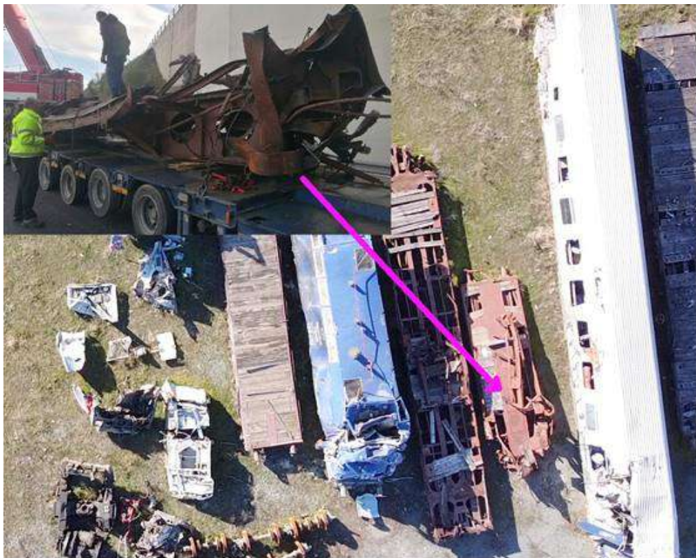
Figure 19. Remains of the first platform that was carrying steel plates.
