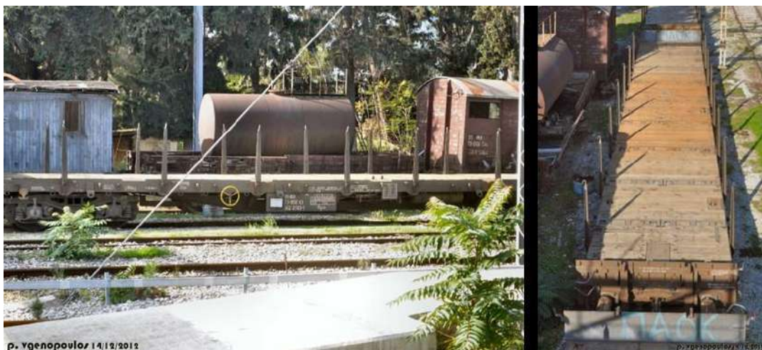
Figure 72. Type of platform supporting the containers (p. vgenopoulos, https://hellas-express.eu/viewtopic.php?f=13&t=69#p361 ).
