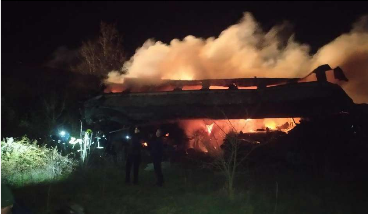
Figure 34. Photo showing the heavy fires in the Restaurant Car area (behind), and on the B2 coach (front, above) (Source: EDAPO).
